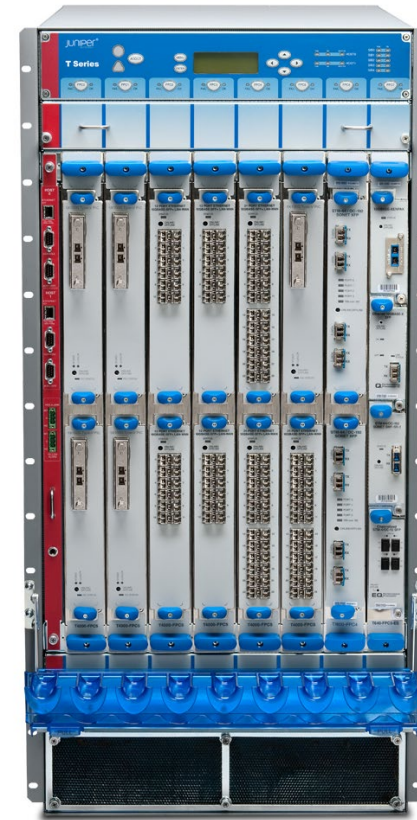
Juniper T4000 Core Router - 3.8 Tbit/s single chassis
