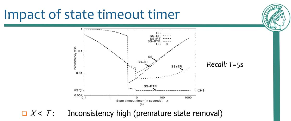
□ X > 2T: Increasing  $X \Rightarrow$  increasing inconsistency for SS, SS+ER, SS+RT (due to orphan state)
